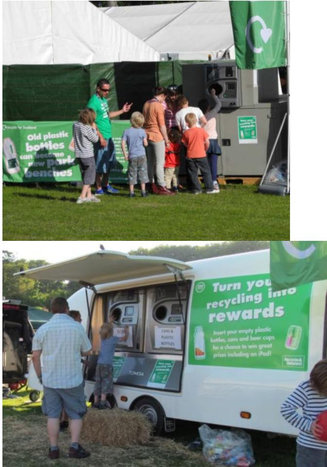
**Figure 2 Single static (above) and twin trailer (below) reverse vending machines**
